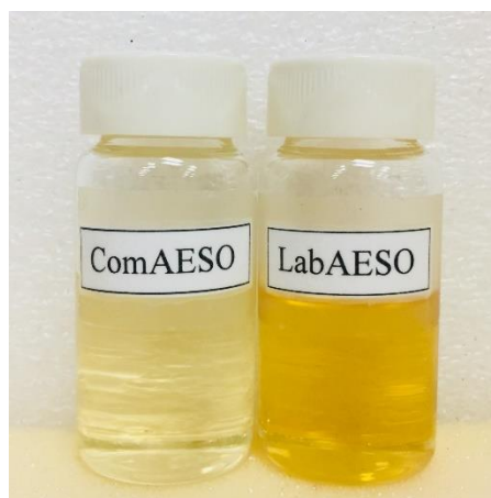
Figure 4.1. Physical conditions of commercial available AESO (ComAESO on the left) and laboratory produced AESO (LabAESO on the right).
